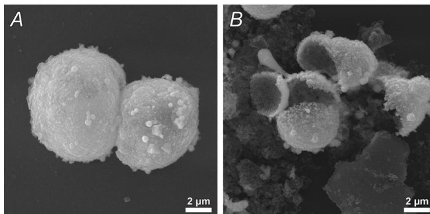
Fig. 3. SEM images of hollow alginate silver microcontainers before and after exposure to electric impulses: *A* – silver alginate microcontainers free of magnetite after exposure to electric impulses; *B* – alginate microcontainers with magnetite nanoparticles immobilized within the shells after exposure to electric impulses
