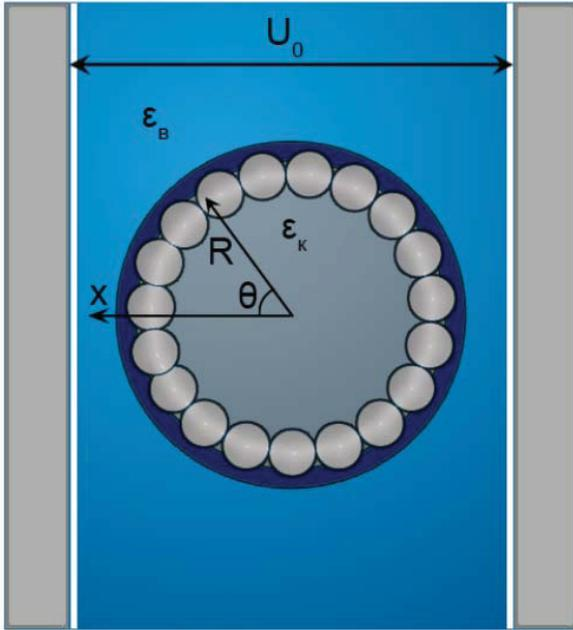
Fig. 2. Scheme of a hybrid alginate microcontainer with magnetite NP immobilized within the shell in the external electric field
