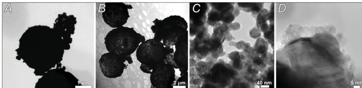
Fig. 1. TEM/STEM images of hollow silver alginate microcontainers: *A* – TEM image of the silver alginate microcontainers; *B* – STEM image of the silver microcontainers after ultrasonic exposure; *C* – STEM image of silver nanoparticles formed within the microcontainer's shell; *D* – TEM image of silver and magnetite nanoparticles within the microcontainer's shell
